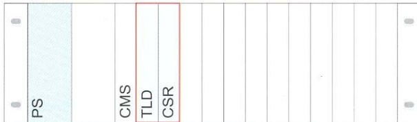
DZ9 /single power supply, single line interface, 2 commands/
